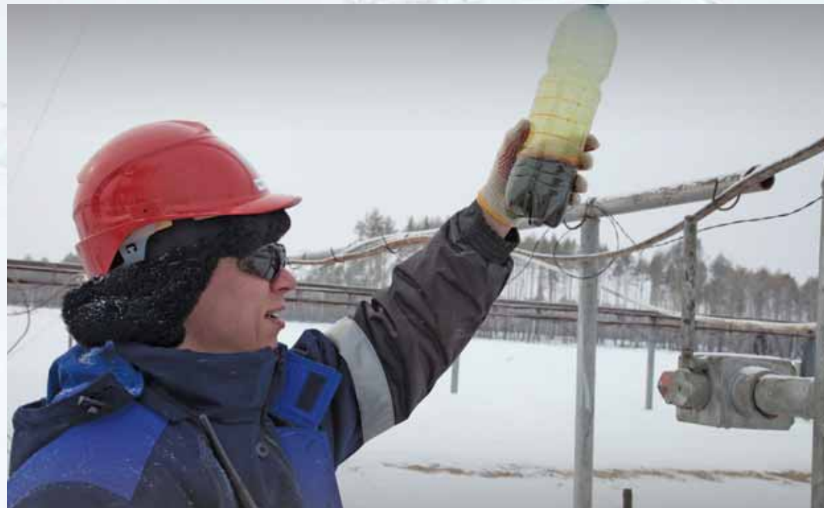
Withdrawal of wellhead samples by oil and gas production operator at Snezhnoye field, Russia
