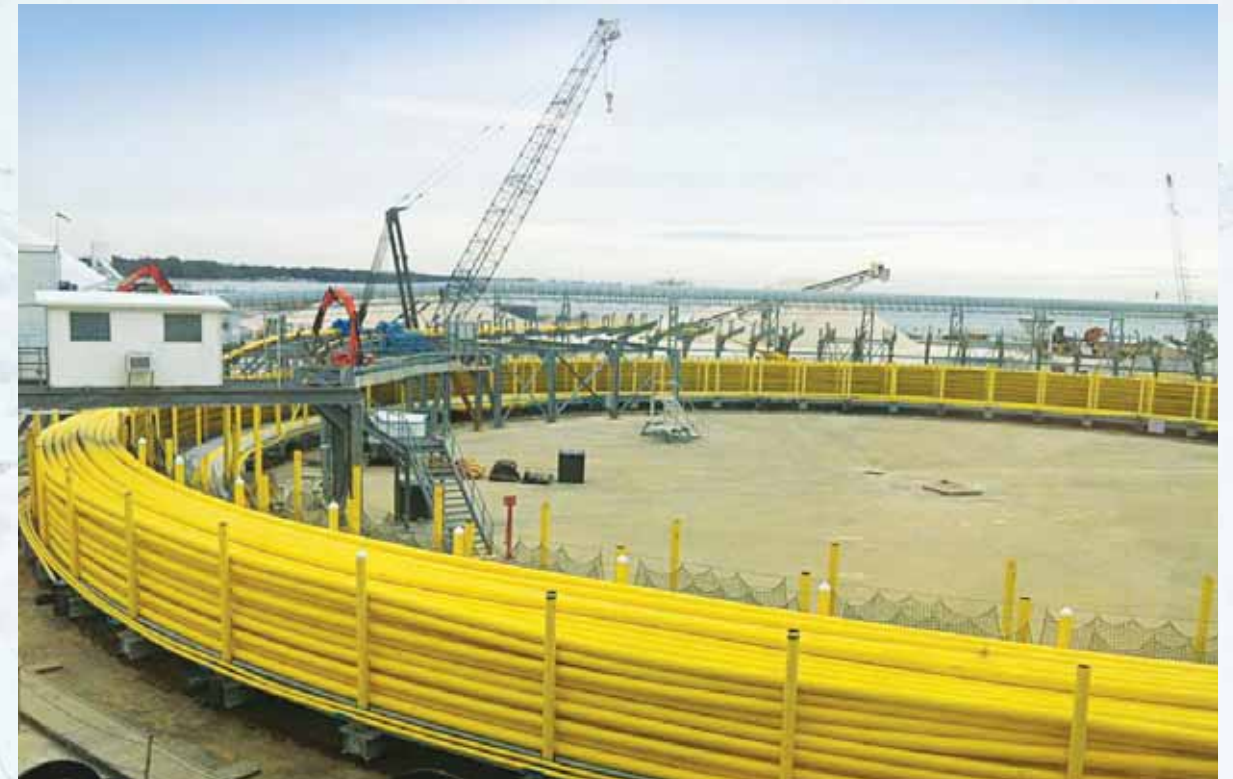
ON-1 & ON-2 dynamic umbilicals on Carousel at Oceaneering Panama City, BC-10 Project
