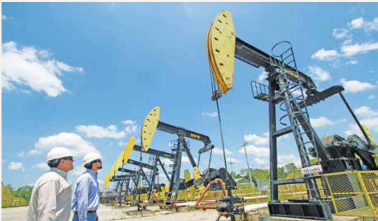
Sucker rod pumps in operation in MECL, Colombia
