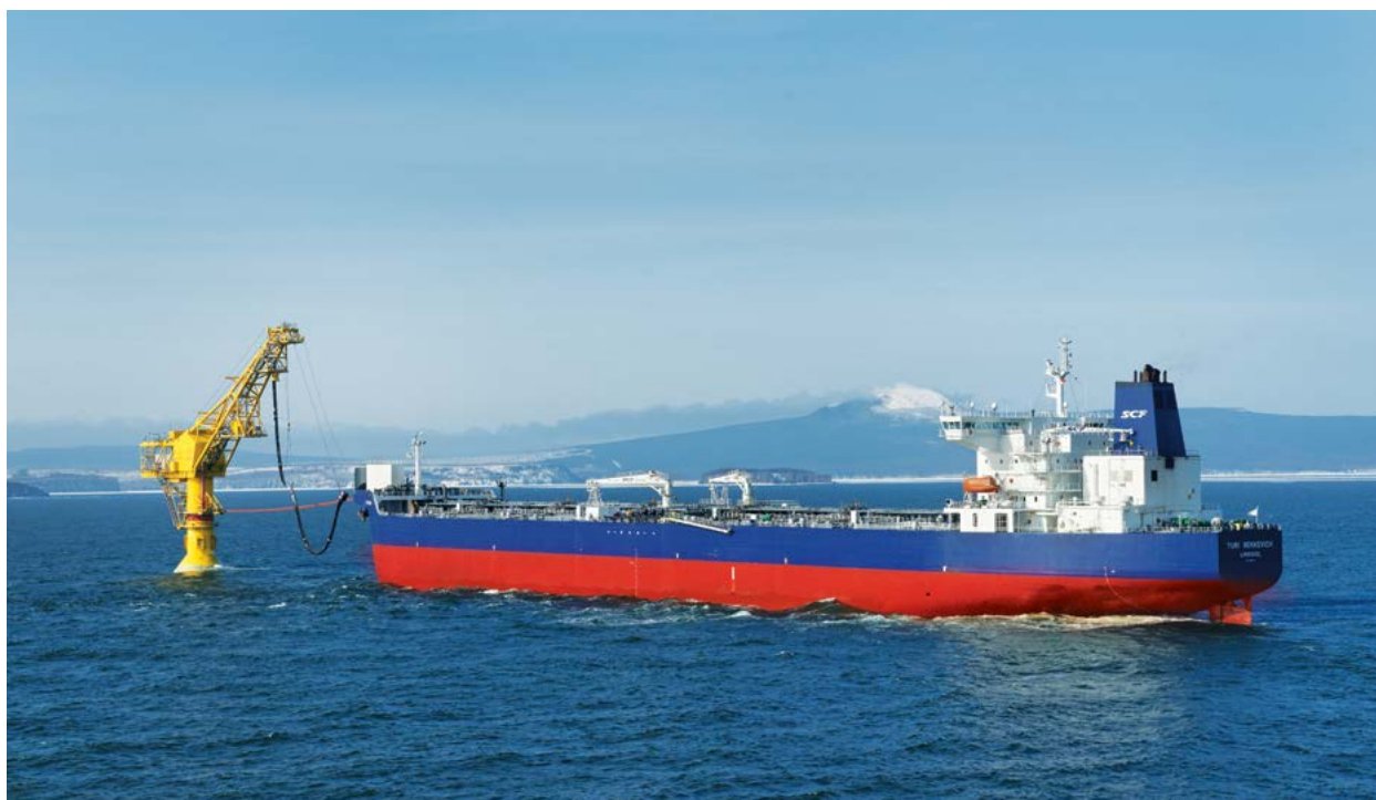
Tankers are loaded using one of the world's largest Single Point Mooring (SPM) which rises 60 meters above sea level
