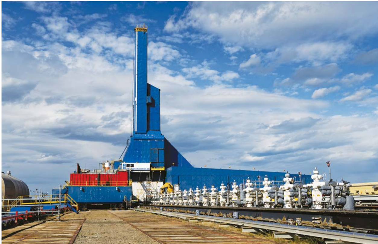
Yastreb Drilling Rig, Chayvo Field, Sakhalin Island, Russia one of the most powerful land rigs in the industry and is designated to drill extended reach wells to offshore targets from land-based locations.
